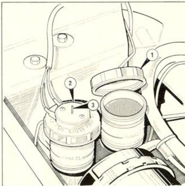
Figure 20 Hydraulic fluid reservoirs
